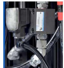
Electronic gear flow meters
